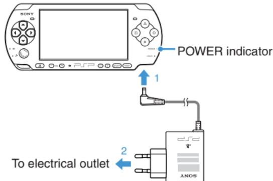
The POWER indicator lights up in orange, indicating that charging has begun. The POWER indicator will turn off when the battery is fully charged.
