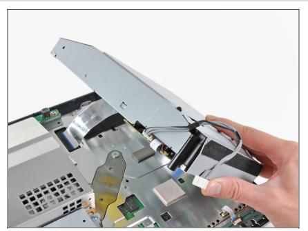
Lift the Blu-ray drive from the edge nearest the power supply and rotate it away from the chassis enough to access its ribbon cable.
