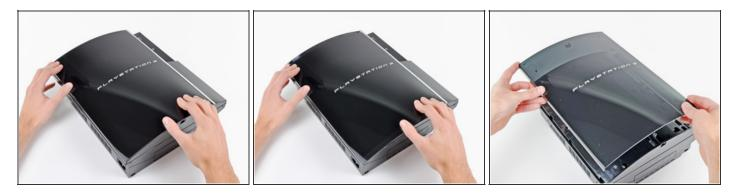
• Pull the smart plate toward the hard drive bay, then lift it off the body of the PS3.
