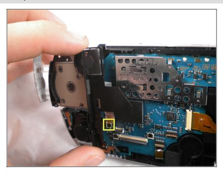
Remove the cable from the connector and remove the entire black piece from the PSP.
