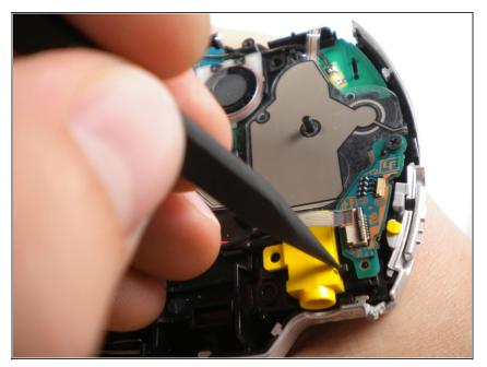
Carefully bend back the black tab holding the power jack in place and start pulling the jack up to release it from this clip.
