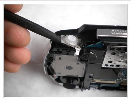
Being careful not to break the ribbon cable, use the spudger to peel the adhesive button of the the 'L' trigger off the PSP.
