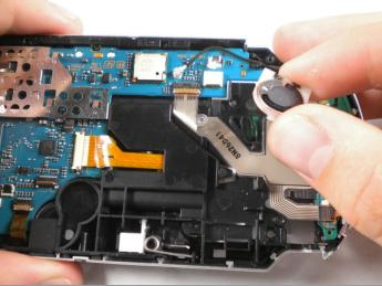
• The speaker is spring loaded, and has a tendancy to pop out and do a few backflips in air when you push the tab. It's pretty entertaining, but be careful not to lose or damage it.
