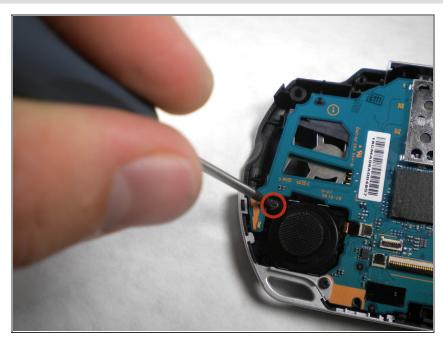
Remove the screw holding the analog stick in place.
