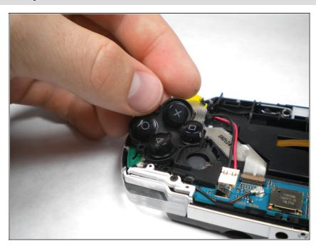
After removing the LCD Screen, the Button Pad should be easily removable.
