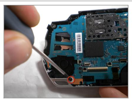
Remove the screw from the bottom left corner of the PSP.
