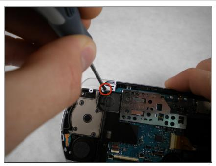
Remove the screw securing 'L' trigger to the PSP.
