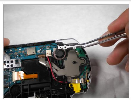
Remove the white plastic piece that holds the 'R' trigger in place.
