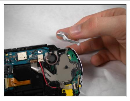
Remove the 'R' trigger from the PSP.
