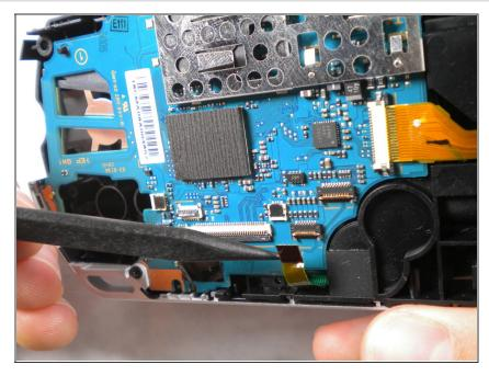
Flip up the lock and remove one last ribbon cable from the bottom edge of the PSP.
