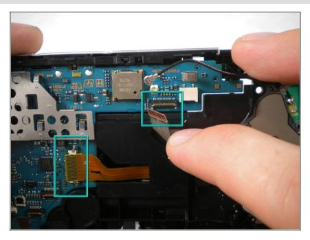
Flip up the locks and remove the two ribbon cables shown.
