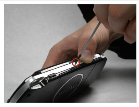
Remove the single screw from the bottom surface of the PSP.
