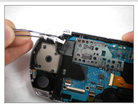
Remove the white plastic piece that holds the 'L' trigger in place.
