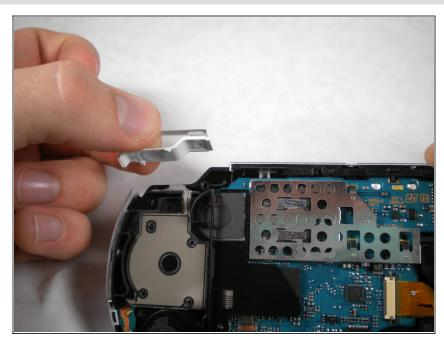
Remove the 'L' trigger from the PSP.
