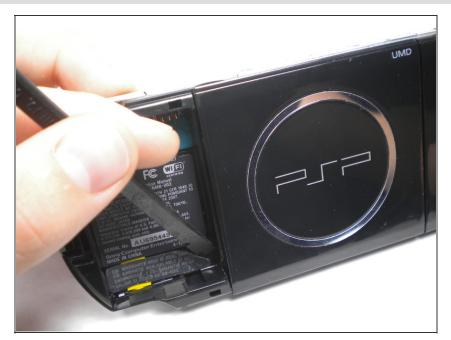
Using a spudger or fingernail, peel back the warranty sticker that is behind the battery.
