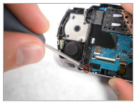
Remove the screw from the bottom left edge of the PSP.
