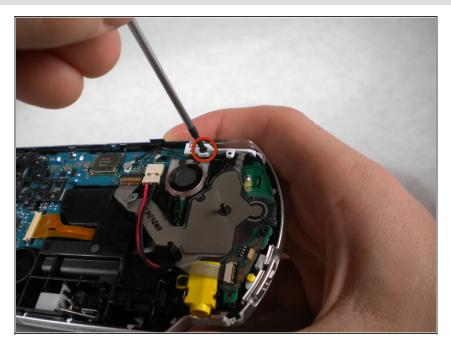
Remove the screw securing 'R' trigger.
