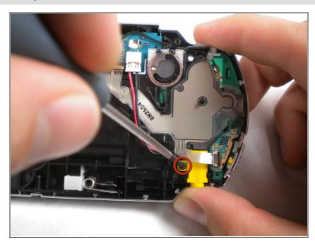
Remove the screw from the power jack.
