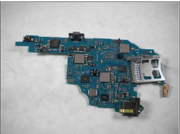
• Pull the motherboard out and remove it from the PSP.
