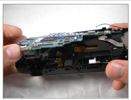
Lift the motherboard up slowly starting from the bottom of the PSP, being careful not to damage the port on top.
