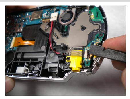
• Flip up the lock and detach the ribbon cable above the power jack.
