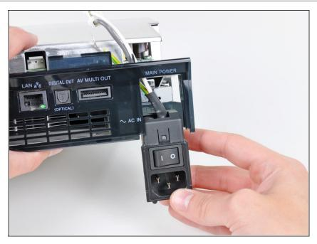
Pull the AC inlet out from the bottom of the rear cover, minding any of its cables that may get caught.
