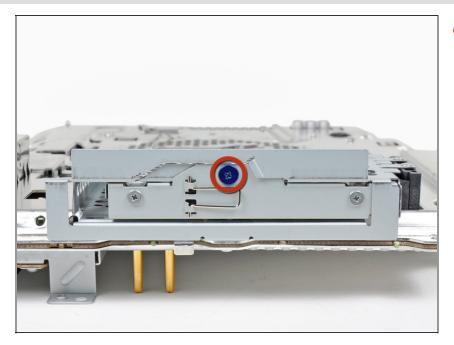
Remove the blue 8 mm Phillips screw securing the hard drive cage to the chassis.
