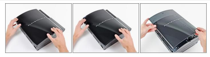
• Pull the smart plate toward the hard drive bay, then lift it off the body of the PS3.
