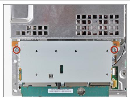
Remove the two 9 mm Phillips screws securing the memory card reader to the chassis.
