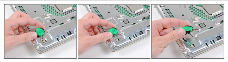
Rotate the PRAM battery slightly counter-clockwise and remove it from the motherboard assembly.
