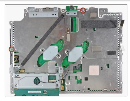
Remove the two 8.3 mm #0 Phillips screws securing the two halves of the motherboard together.
