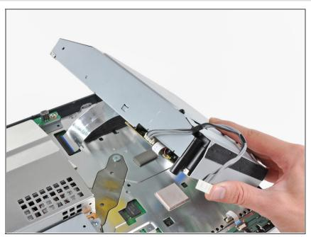
Lift the Blu-ray drive from the edge nearest the power supply and rotate it away from the chassis enough to access its ribbon cable.
