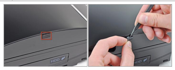
• Use the tip of a spudger to remove the black rubber screw cover from the side of the PS3.
