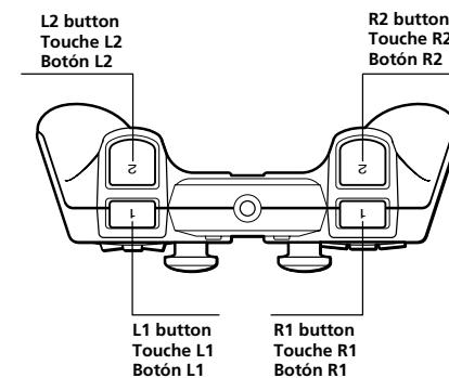
\* The R3 button and the L3 button function when the stick is pressed.
