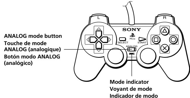
Check the software package and switch to the appropriate mode for use. Note however, that some software applications make this mode change automatically, so manual adjustment is not possible. In such cases, the ANALOG mode button is overridden by the software. For details, refer to the software manual.
