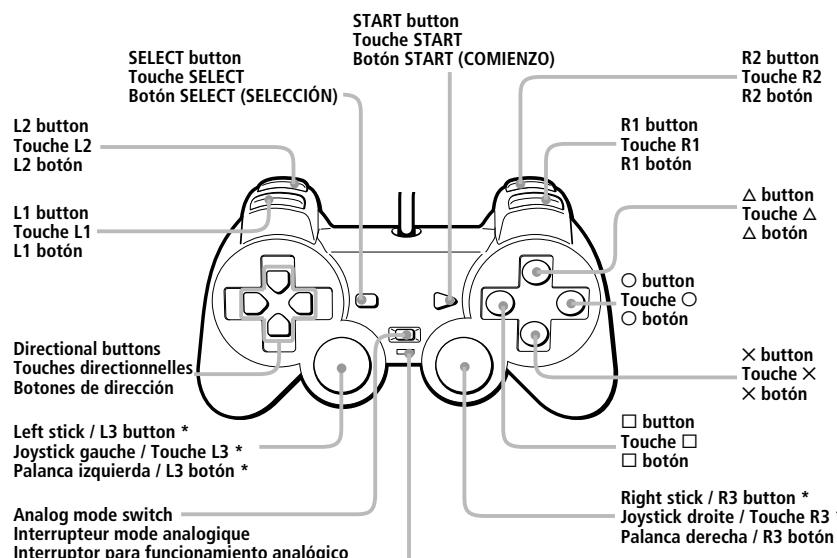
\* The R3 button and the L3 button function when the stick is pressed.
