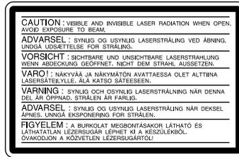
This label is located on the protective housing of the CD/DVD unit inside the enclosure.
