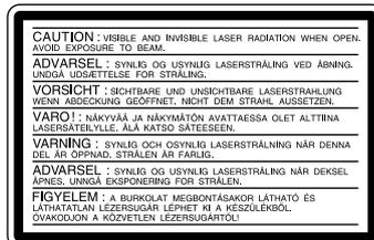
This label is located on the protective housing of the CD/DVD unit inside the enclosure.
