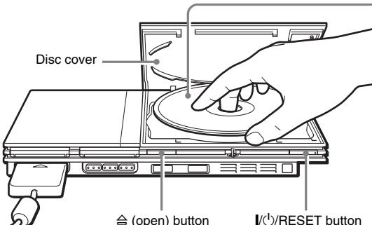
Place the disc in the console with the label side facing up.
