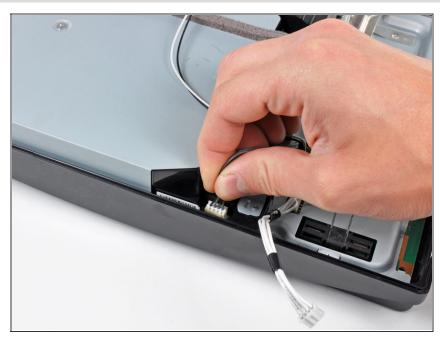
Pull the Blu-ray power cable straight up to lift its connector out of the socket on the Blu-ray drive.
