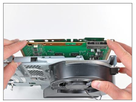
If necessary, gently pry the motherboard off the top shield near the heat sink and its shroud.
