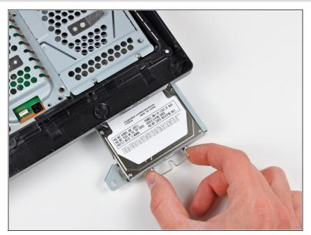
Using its attached metal handle, pull the hard drive out of its bay.
