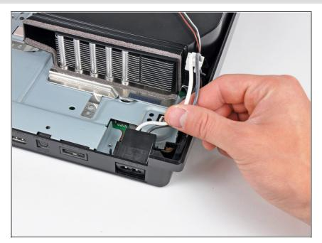
Pull the AC-In cables upward to remove the AC inlet from the lower case.
