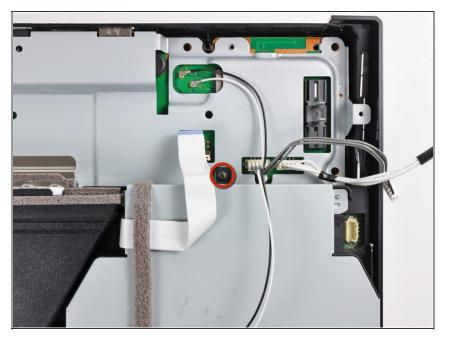
Remove the single 9.5 mm Phillips screw securing the Blu-ray drive to the lower case.
