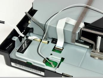
If present, remove the pieces of tape securing the cables to the body of the Blu-ray drive.
