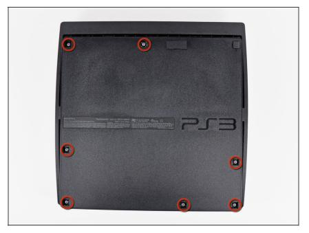
Remove the seven 37 mm Phillips screws securing the top cover to the lower case.
