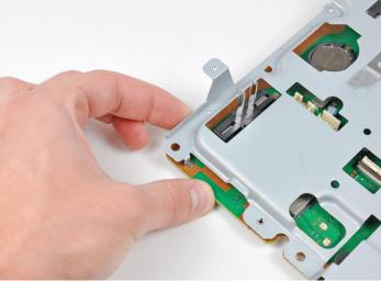
• Gently press the board away from the top shield assembly near the fan connector and the corner of the board near the wireless sockets.
