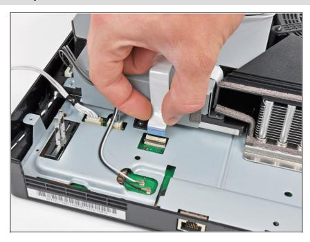
Pull the Blu-ray ribbon cable straight up and out of its socket.
