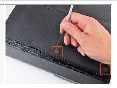
• Use the flat end of a metal spudger to pry up the seven screw covers around the edge of the lower case.
