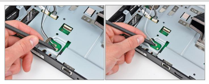
• Use the flat end of a spudger to pry both antenna connectors up from their sockets on the motherboard.
