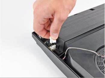
• Squeeze the AC inlet connector's locking mechanism and pull straight up to disconnect it from the power supply.
