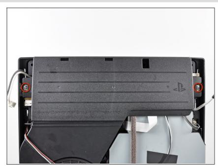
Remove the two 7.6 mm Phillips screws securing the power supply to the lower case.
