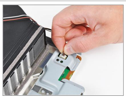
Pull the fan cables straight up to lift the fan connector up and out of its socket on the motherboard.
