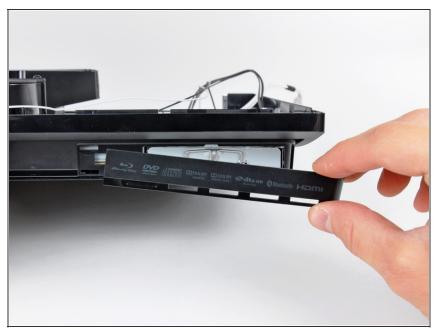
Slide the hard drive bay cover toward the right side of the lower case, then pull it away from the front edge to remove it from the PS3.
