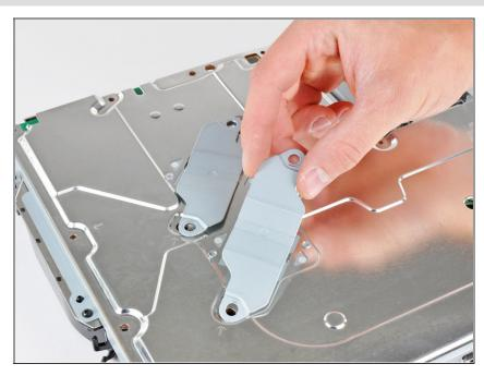
Remove the two heat sink clamps from the bottom of the motherboard assembly.
