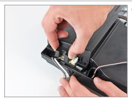
Lift the power supply upward from its left edge as viewed from the front of the PS3.
