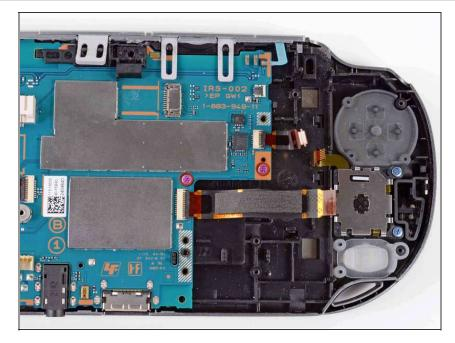
Using a Phillips #00 screwdriver, remove the two pink, 4.4mm screws securing the motherboard.
