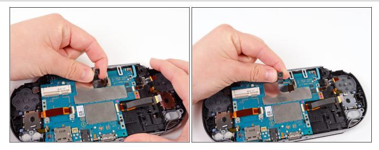
• Carefully lift and remove the camera, sliding the flex cable out of the open connector socket.
