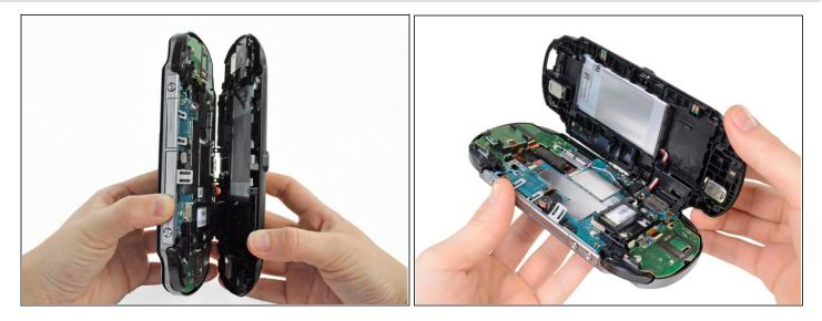
• Gently separate the two cases, minding the battery and the touch screen controller connectors holding the two cases together.
