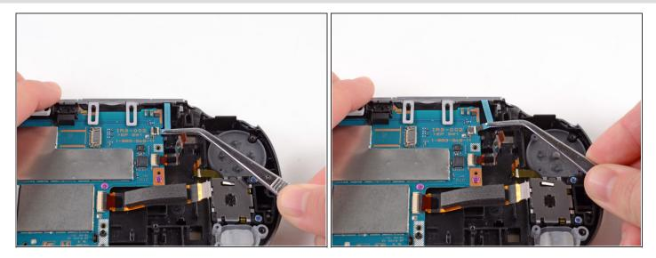
• Using tweezers, gently pull the blue power flex cable out of the socket; rest it out of the way.
