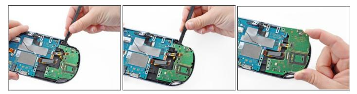
• Starting from the upper left corner, use a spudger to pry up and remove the left button board.
