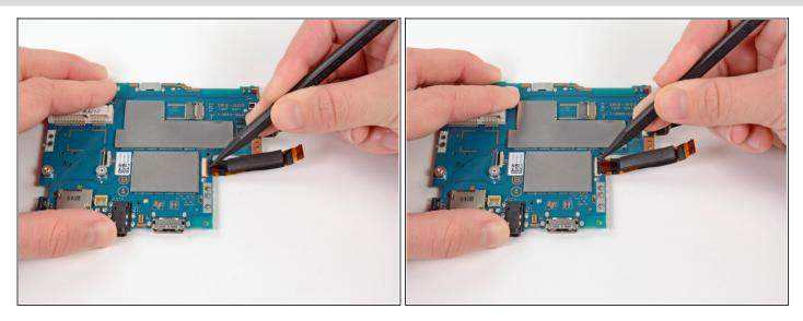
• Release the tab on the large ZIF connector on the right side of the motherboard by lifting the tab with a spudger.
