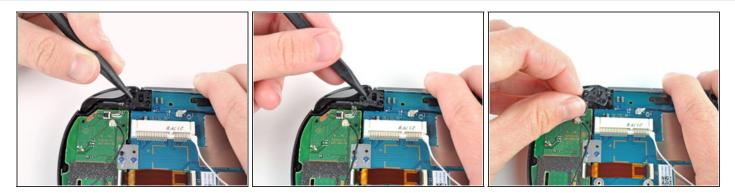
• Pry up the right shoulder button casing with a spudger and set it aside.
