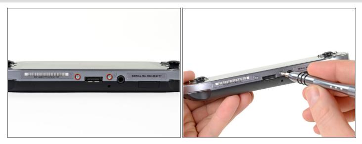
Remove the two 5.4mm Phillips #00 screws on the top of the device near the charging port.
