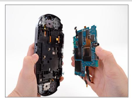
Completely separate the motherboard from the case.
