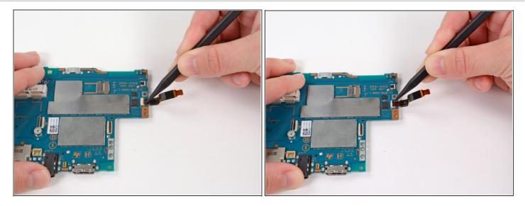
• Using a spudger, release the small ZIF connector on the right side of the motherboard.
