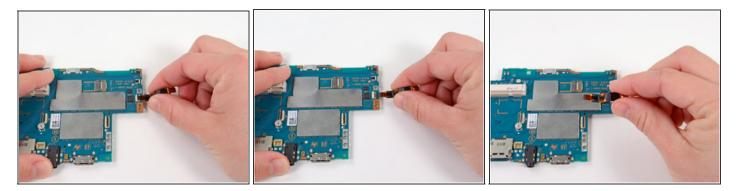
• Gently pull the flex cable out of the small ZIF connector, and remove it.
