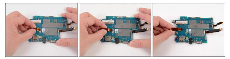
• Gently pull the flex cable out of the ZIF connector, and remove it.
