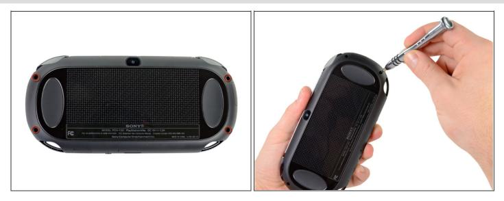
• Using a Phillips #00 screwdriver, remove the four 6.4mm screws on the back casing.
