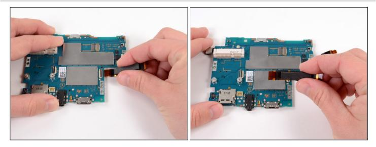
• Gently pull the flex cable out of the ZIF connector, and remove it.
