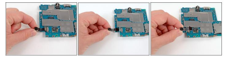
• Gently pull the rear camera out of the connector and remove it.
