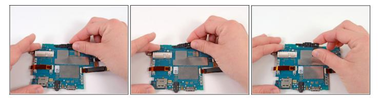
• Starting at the right side, gently lift and remove the black casing that once held the camera.
