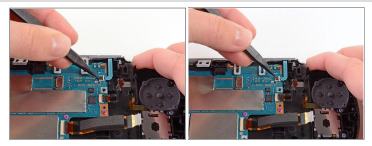
• With the help of a spudger, lift and release the tab on the blue flex cable socket.
