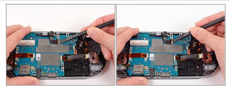
• Release the camera flex cable socket by prying up on the tab with a spudger.
