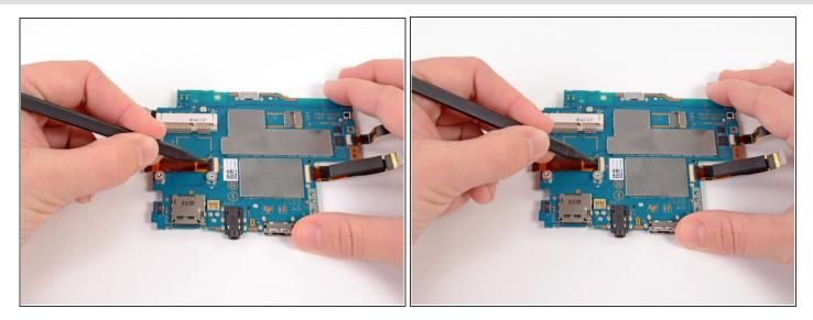
• Using a spudger, release the tab on the ZIF connector located above the two screw posts where the wireless card once was.
