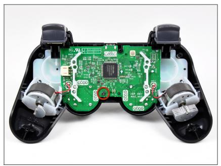
Remove the single 7.2 mm Phillips screw securing the motherboard to the front cover.
