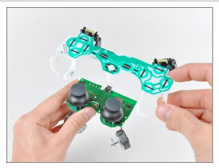
• Lift the input board assembly off the motherboard.
