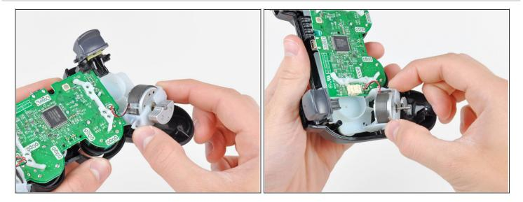
Pull the vibration motor retainers away from the front cover to dislodge the motherboard assembly.
