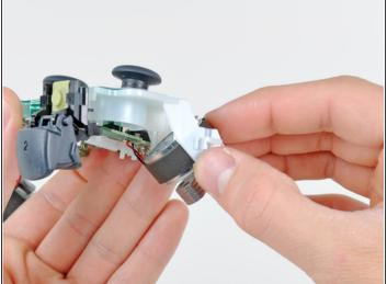
• Carefully push the two vibration motors out of the input board frame.
