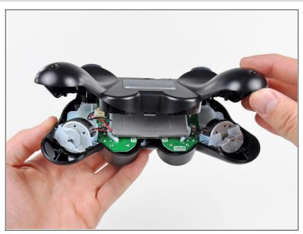
Slightly lift the lower edge of the rear cover away from the rest of the controller.
