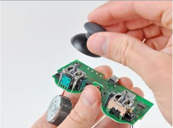
Pull both analog stick covers straight up off their joystick posts attached to the motherboard.
